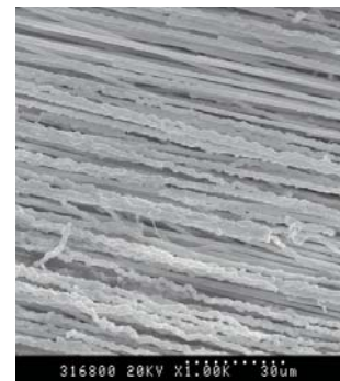
Fig. 4. Layers of nanowires in specimen S4 with growth time of 10 minutes: flexural nanowires are found on top of smooth nanowires layers.
